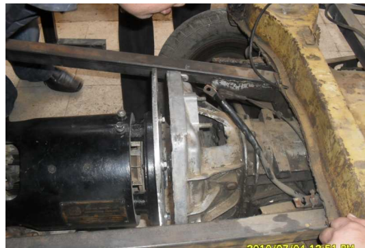
Figure (8) shows the assembly of electric motor with the transmission system. Rubber pads are placed beneath every mount to isolate some of the vibrations. A brace was added to help supporting the electric motor. The figure below showing the electric motor used in our vehicle and how it connected and assembled with the transmission parts.
