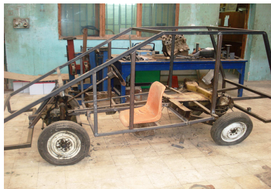
Figure (2) the assembly of frame and chassis for the electric vehicle (side view).
