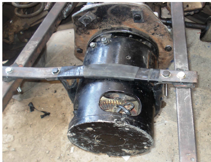
Figure (9) shows the mounting of the electric motor.
